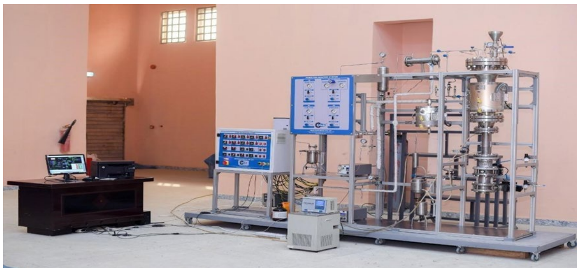
Figure 2: The Integrated Pyrolysis and Fixed Bed Reactor System at the National Research Institute for Chemical Technology, Zaria.
